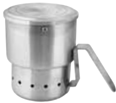
Spring Heating Element 220-240V, 400Watts Size (Ø)110×(H)135mm After Compress (H)105mm
